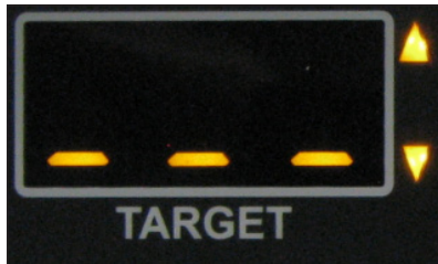
Figure 3.3.1e Both up and down Arrows display in Stationary All Mode when front or rear antenna is selected.
