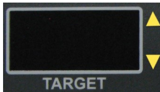
Figure 4.2.1e TARGET Direction indicator lights
