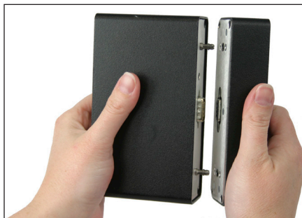
Figure 2.1a Separating the computer/display unit.
